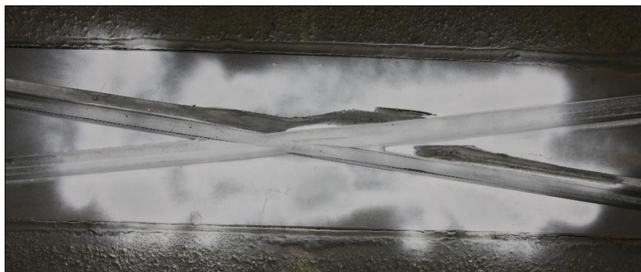
Fig. 2 – Riding on the top of the crossing (without contact with the groove, typical for a deep groove)
