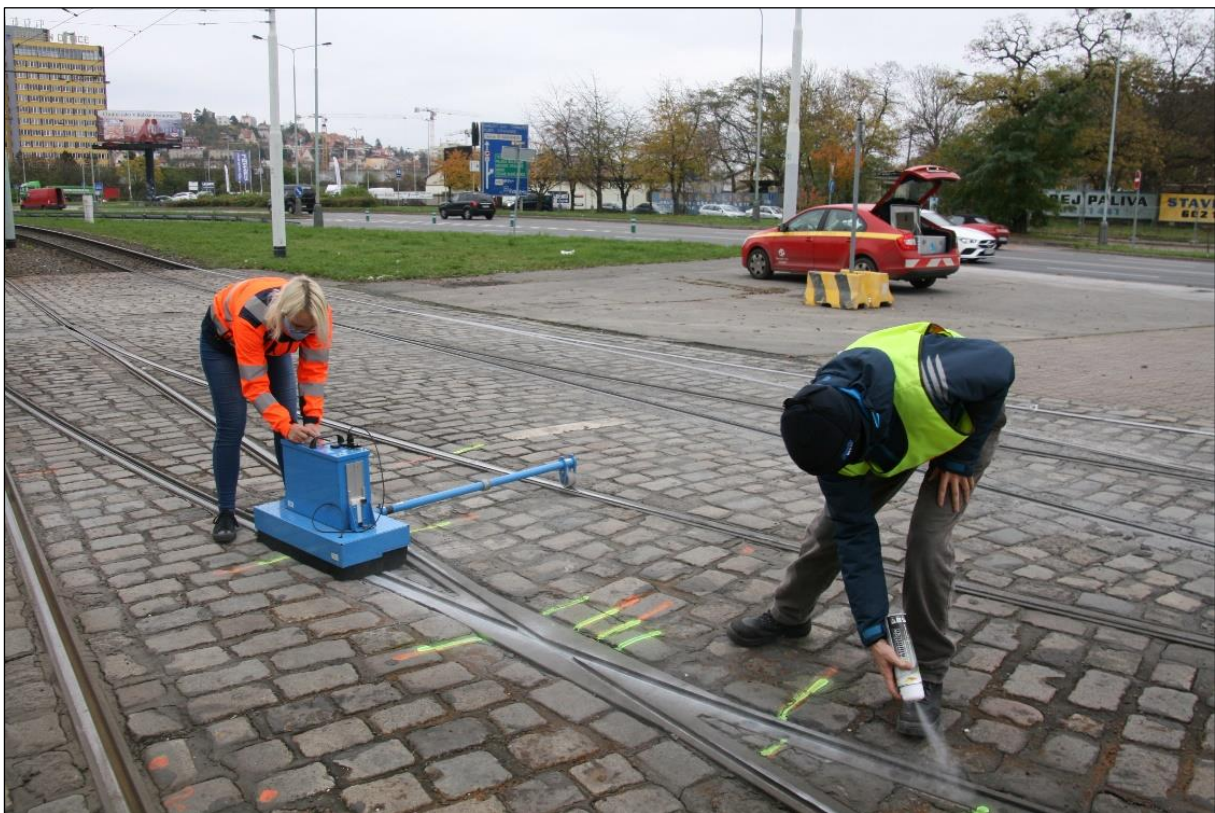
Fig. 5 – Measurement of the cross-section profile of crossing grooves
