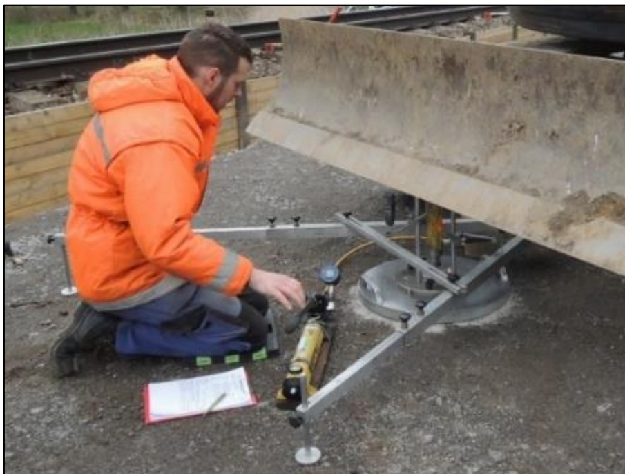
Fig. 1 – Performing the SPLT according to the French methodology
